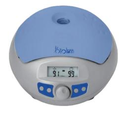
The BL-D2012 Microcentrifuge is a versatile tool widely used in molecular biology laboratories. With a maximum speed of 15000rpm (15100×g), it facilitates plasmid extraction, nucleic acid purification, pre-sequencing processing, and various biochemical analyses. Its quick pulse operation, brushless DC motor, and safety features ensure efficient and safe operations.
