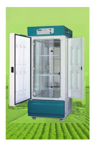
PGC-Series 3-Side Illumination Plant Growth Chamber provides reliable controlled climatic condition of temperature, humidity, lighting and CO2 concentration(Optional). Ideal to growing plant, plant tissue culture or any other laboratory experiments needs controlled climatic simulation. Various choice of capacity from 200L ~ 864 L for tissue culture and plants growing. Light bank on the 3- side with fluorescent lamps provides light intensity up to 30,000 LUX.
