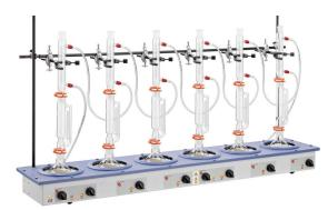
A Soxhlet extractor is a piece of laboratory apparatus. It was originally designed for the extraction of a lipid from a solid material. Typically, Soxhlet extraction is used when the desired compound has a limited solubility in a solvent, and the impurity is insoluble in that solvent. It allows for unmonitored and unmanaged operation while efficiently recycling a small amount of solvent to dissolve a larger amount of material.
