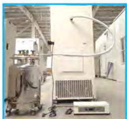
LN 2 /CO 2 backup system
