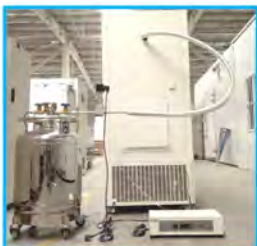
LN2/CO2 backup system
