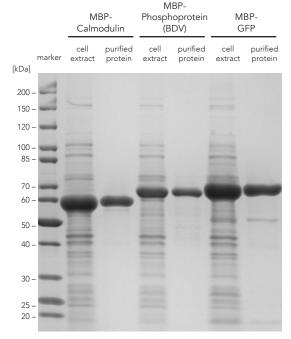
The MBP-Spin™ Protein Miniprep Kit purifies high-quality MBP-tagged proteins directly from a spin-column. N-terminal MBP-tag fusion proteins were expressed in *E. coli* cells, and the cell extracts as well as the proteins purified using the MBP-Spin™ Protein Miniprep Kit were analyzed by SDS-PAGE on a 4-20% gel and stained with InstantBlue™; (MBP-Calmodulin 55 kDa, MBP-BDV-Phosphoprotein 65 kDa, MBP-GFP 69 kDa).
