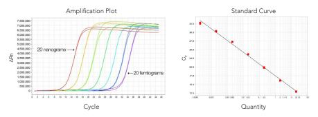
Reliable standards for the quantification of bacterial DNA. Bacterial DNA Standards (measured in duplicates) comprise a 10-fold dilution series ranging from 20 ng to 20 fg.
