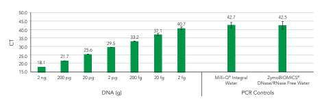
Amplification of the 16S rRNA gene can be quantified down to 2 femtograms (fg) of bacterial genomic DNA. Quantified non-template controls, including Milli-Q and ZymoBIOMICS® DNase and RNase-free water, demonstrate the minimal bacterial DNA contamination.
