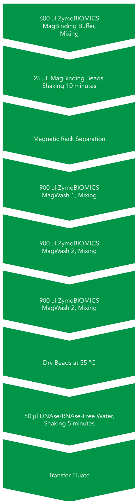
Figure 5: Workflow for the ZymoBIOMICS-96 MagBead DNA Kit
