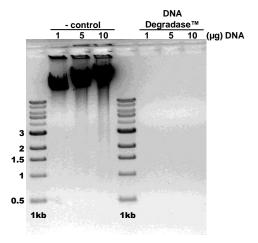
**DNA Degradase<sup>TM</sup> Efficiently Degrades DNA:** 1 µg, 5 µg, and 10 µg of  $\lambda$  DNA incubated with 1 µl (10 U) of DNA Degradase<sup>TM</sup> in 25 µl reaction volume (see *Standard Reaction Setup*) and incubated at 37°C for 1 hour.
