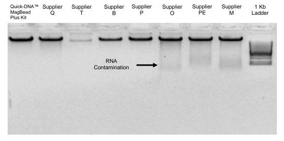
High DNA Yields With RNA Removal Technology. 200 µl human blood was processed using the Quick-DNA™ MagBead Plus Kit compared to various competitor MagBead purification kits (n=2). Input DNA was analyzed in a 1% (w/v) TAE/agarose/EtBr gel (shown above). The gel electrophoresis was prematurely paused to check for RNA contamination.
